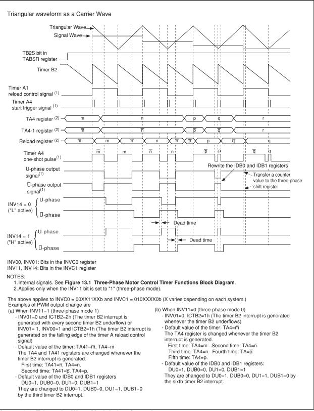
Figure 13.9 Triangular Wave Modulation Operation
